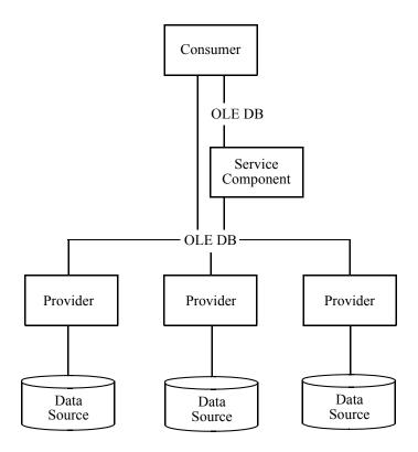
OLE DB provides a common set of object-oriented interfaces, which is the "wiring" the various OLE DB components need to work seamlessly together. These cooperating components produce and consume data that is exposed from data sources in the form of rowsets. The rowset interface guarantees that data can be used across the enterprise in a consistent and uniform way, regardless of its original source.
