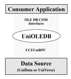
UniOLEDB exposes the data in a UniData or UniVerse data store. It uses UCI, which is an application programming interface (API) that UniOLEDB uses to access data in UniData and UniVerse databases. UCI uses UniRPC, a library of calls developed by IBM, to implement remote procedure calls. UniOLEDB passes the results back to the consumer application in the form of a rowset.
