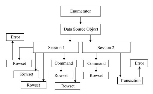
This example illustrates the standard relationships between the various objects. The enumerator identifies a data source object for a data source. The data source object generates two sessions, each representing a connection to the data source.
