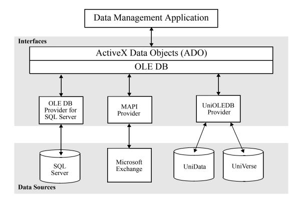
In this example, ADO functions as an application-level interface to OLE DB. ADO is not dependent on any particular programming tools or languages. OLE DB provides the underlying, system-level interfaces for data access. The ADO interface is optional. The data management application could use a different application-level interface, such as an SQL Server query processor, to access data. It also could use the OLE DB interfaces directly.
