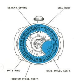
A finger attached to the date wheel assembly engages with and moves the date ring. A detent spring holds the date ring in position and also aids in moving the date ring. A pinion attached to the hour wheel (No. 2558 on the exploded view) engages with the date wheel assembly.
