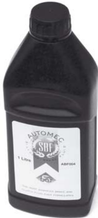
053.018 Silicone brake fluid 1 litre, for extended use. It is silicone based, it won't absorb water that can cause corrosion. do not mix with conventional fluids
