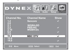
4 Press ▲ or ▼ to highlight the channel you want to hide (the default is to show the channel), then press ENTER to remove the check mark from the channel.
