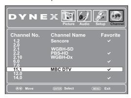
5 Press ▲ or ▼ to highlight the channel you want to add to the favorite list, then press **ENTER** to mark the channel. A check mark appears if the channel is added to the list. The check mark disappears if you delete the channel from the list.
