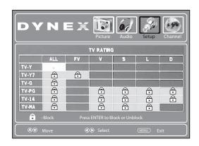
8 Press ▲ ▼ ⋖ or ► to highlight the rating you want to block, then press ENTER. A lock symbol appears when a rating is blocked.
