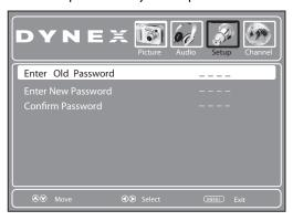
**6** Press the number buttons to input old password, then input a new password. On the next line, enter the new password again to confirm it. The *Parental Controls* sub-menu reopens.
