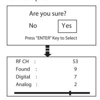
5 Press o or to select Yes, then press ENTER to start the scan. A progress box shows the progress of the scan.
