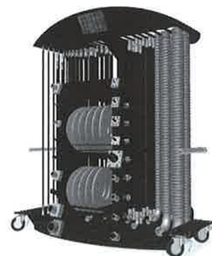
The custom hose and component rack with connection chart.
